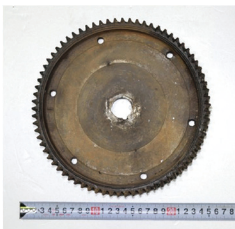
Fig.5 Dismantle d Flywheel
