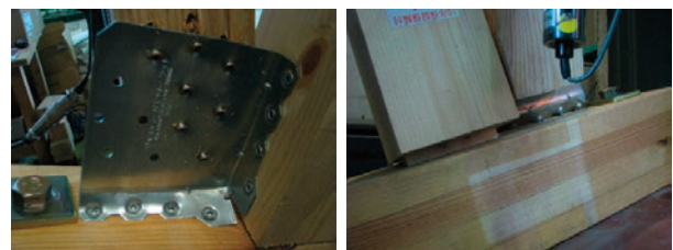
Photo4 Failure condition of J-m-1
