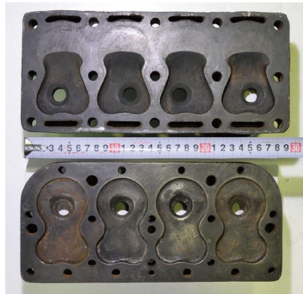
Fig.11 Combustion chamber of Datsun type 17 and Austin seven
