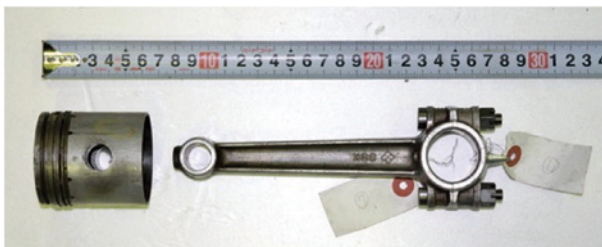
Fig.4 Dismantle d piston and connecting rod
